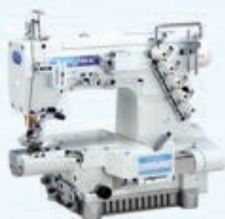
CT9713-0-356M 包縫骨壓縫 (倒骨式、包縫骨寬度3.0m.m. 以內) Overlock Seam Covering (Folding Over, Overlock Seam Width Under 3.0m.m.)
