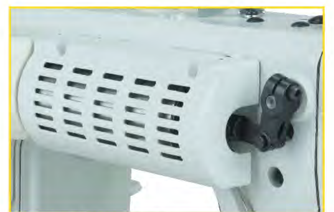
前置背掛式自動抬壓腳 Front backside automatic foot lifter
