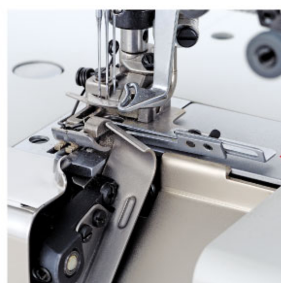
上送帶 / 鬆緊帶串縫 Top feeding tape / Elastic tape Attachin
