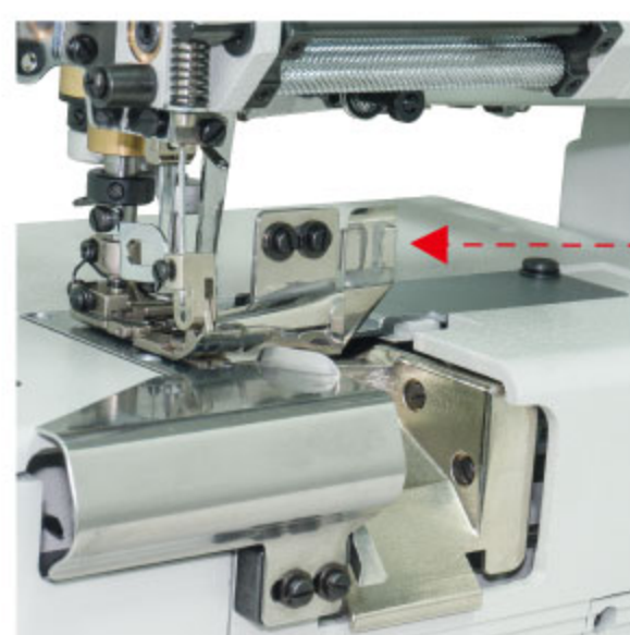
上送帶 / 細滾邊 Top feeding tape/ Fine tape binding
