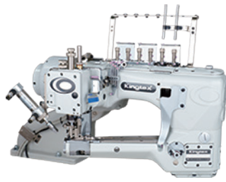
NTD77 / TC026 FEED-OFF-THE-ARM MACHINE FOR FLAT SEAMING
