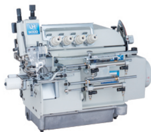
UHU9304/TR025 Automatic chain cutter device direct-drive cylinder bed top feed overlock fitted with labor-saving rib folder
